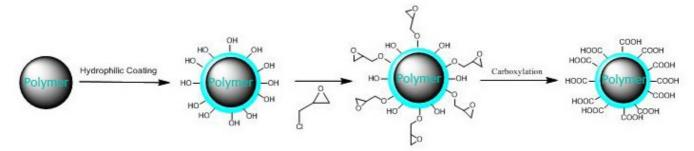
The structure of carboxyl treated magnetic polystyrene microspheres is typically sandwich type. The inner core is monodisperse polymer microspheres. Magnetic oxide layer is in the middle between uniform polymer microspheres and the outermost layer which is hydrophilic and hydroxyl functionalized polymer layer. By carboxylation, hydroxyl groups convert to carboxyl groups.
